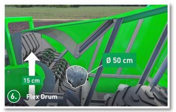
The lifting drum's power transmission is mounted along the drum frame, allowing the frame and the entire lifting drum to yield upwards, which makes it possible to lift stones with diameter 50 cm/20 in.
