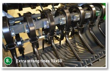
All tine sizes give way sideways to prevent blockages. That's why rotation backwards is not required. 13x50mm/0.51x2in tine is much more durable than standard 12x45mm/0.47x1.8in tine and this lengthens the maintenance interval.
