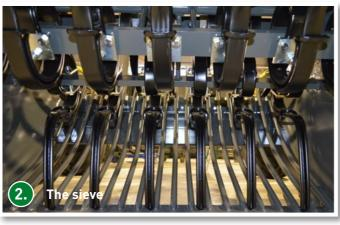
The welded sieve is made of special steel and is available with different spacings (40,50,70mm) The farmer can choose what size stones to pick up and what size to leave in the field. The tines run between the sieve bars the entire length thus keeping the sieve clean and preventing jamming of rocks.
