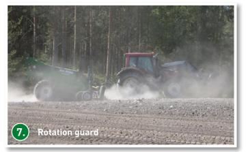
When Kivi-Pekka is operated in dusty conditions, the rotation guard monitors the operation of the rotors, the lifting drum and main drive PTO shaft. An auditory alarm in the tractor cab alerts the operator if a component has stopped turning.
