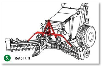
The lifting action is achieved with hydraulic cylinder, which raises both rotors simultaneously. The rotors are locked into the top position with mechanical locks. The PTO shafts can be connected during lifting
