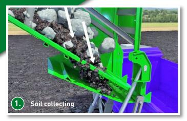
The back of the machine is grated which cleans the dirt from the rocks when the container is dumped. This allows the rocks to be used for landscaping, construction or road construction.
