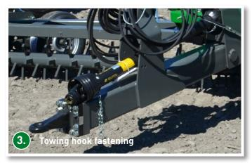
The stone picker has Scharmuller's towing eye as standard. It is possible to install ball coupling as accessory.
