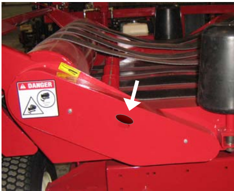
Figure 5.3 Other lubrication 2 (through the hole in the guard)
