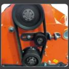
Adjustable axial floating belt tensioner (ensures durabilitylimiting the power dissipation inheat
