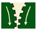
Flat groove design wears better and creates less dust. Primarily used for cracking, crimping, or flaking grain.
