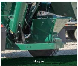
Supplement Hopper Rear-mounted concentrate hopper with built-in sack cutter for easier access.
