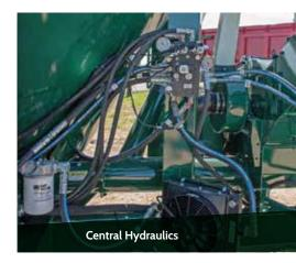
**Centralized Hydraulics** Easier adjustment with central hydraulic bank with easy-toread pressure gauges for better
