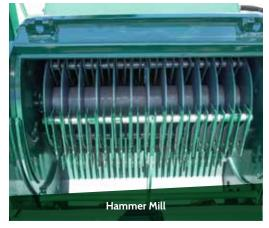
**4-way Reversible Hammers** The 26-inch hammer mill boasts 96 4-way reversible hammers for long use and easy replacement.
