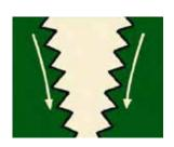
Sharp tooth design offers higher capacity and is fit for grinding powder processing.
