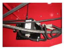
Figure 62 - The receiver of the remote steering
