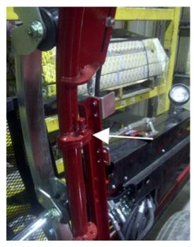
Figure 54 – Adjusting the tension of the outside hoop
