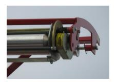
Figure 37 – The gears of the stretcher system
