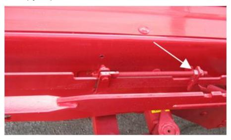
Figure 46 – Adjusting the pusher trigger for round bales (nuts)
