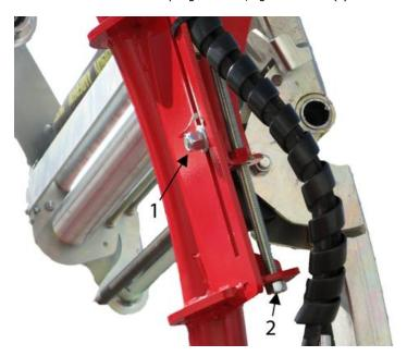
Figure 55 – Adjusting the hoop drive wheel
