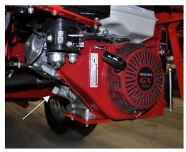
Figure 6 - Engine oil cap location
