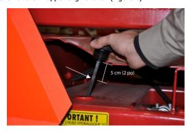
Figure 5 - Oil in Hydraulic oil tank
