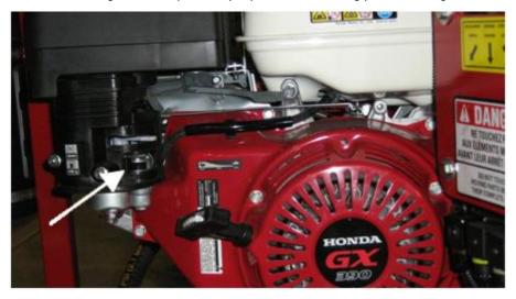
Figure 4 - Closing the fuel valve
