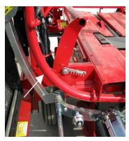
3. Once the tension has been adjusted correctly, insert the spacers provided by Anderson to fill in the spaces on the inside hoop plates.
