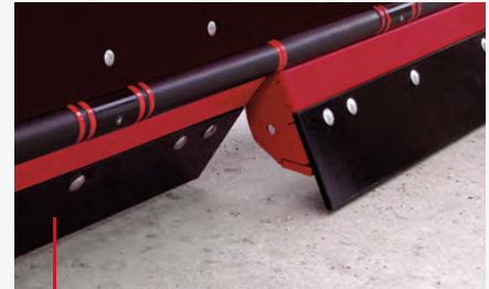
High clearance split trip-edges operate independently of one another, reducing stress and twisting forces on the plow.
