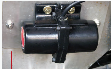
Optional vibrator helps keep material moving.
