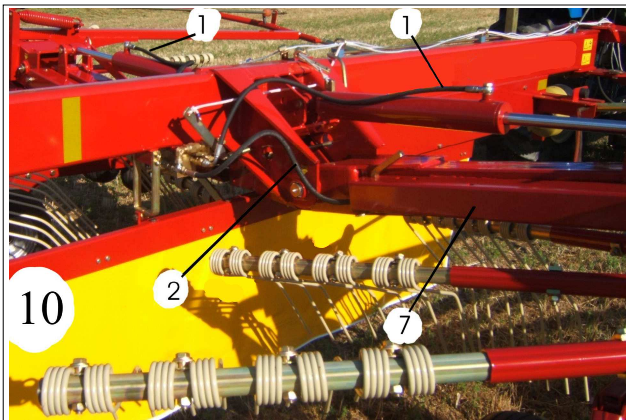
Fig.10/11 Assemble the accessories in the central area: hydraulic hoses (1for lift and 2 for extension), arm extension adjustment housing (7), flow divider (4), valve extension (5), valve control lever (3), spring lever (6), bracket (8)
