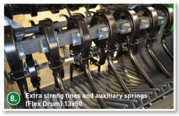
All tine sizes give way sideways to prevent blockages. No backwards rotation is hence required. The 13x50(1/2"x2") Flex Drum tine is particularly durable and contributes to extended maintenance intervals. All tines are fitted with auxiliary springs and suspended with rubber buffers.
