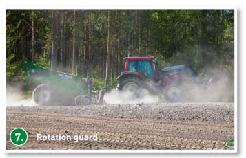
When operated in dusty conditions, the rotation guard monitors the operation of the rotors, the lifting drum and the main drive PTO shaft with sensors. An auditory alarm in the tractor cab alerts the operator if any of these stops turning.
