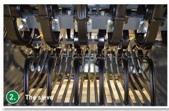
The welded sieve is made of special-alloy steel and is available with different spacings. The tines run between the sieve bars the entire length, thus keeping the sieve clean and preventing jamming of rocks.
