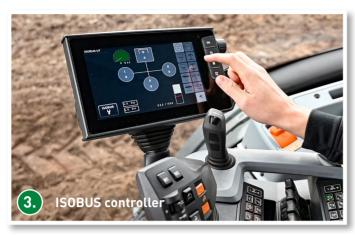
The stone picker equipped with Isobus control measures the working depth with an ultrasonic sensor and adjusts the depth automatically. If the stones get jammed, the machine automatically relieves the rotors and raises the Flex Drum lifting drum.
