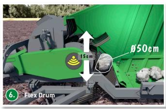
The lifting drum's power transmission is mounted along the drum frame, allowing the frame and the entire lifting drum to yield upwards, which makes it possible to lift stones 50 cm in diameter.
