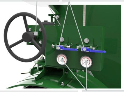
Individual pressure gauges monitor the braking force applied to each wheel.
