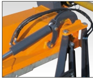
Rotation joint on self lubricating bushing.
